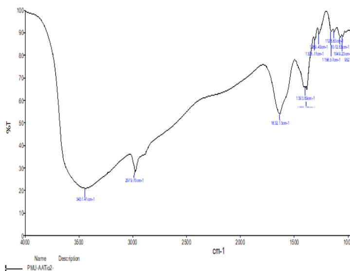
Fig : 2 FTI spectra of the SiO<sub>2</sub> -TiO<sub>2</sub>-ZnO Nanocomposites
