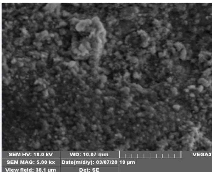
Fig : 1 SEM images of TiO<sub>2</sub>/ZnO/ SiO<sub>2</sub> nanocomposites at 5000x
